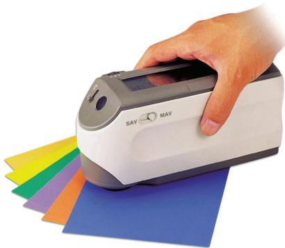
To utilise the DosiXpress™ system, the ColorMatrix customer uses a hand held Spectrophotometer, typically a "Konica Minolta CM-2600d", connected to their pc to measure the color values of a sample they wish to match to. The system then evaluates this match against the colorant palette available from ColorMatrix and offers up to 50 formulation options to the customer to choose from.
