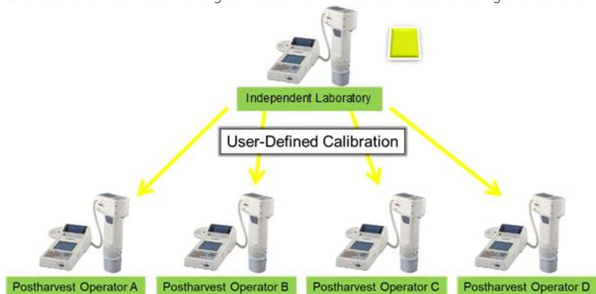
In New Zealand, when the kiwifruit industry players either receive a new CR-400 or a corrective unit back from recalibration/repair, they need to send the unit to the independent laboratory appointed by the kiwifruit exporter first and the laboratory will perform the user-defined calibration on the unit using specific color tiles before they commence the usage of the instrument. This common practise is to ensure close inter-instrument agreement of CR-400 used in the kiwifruit industry.
