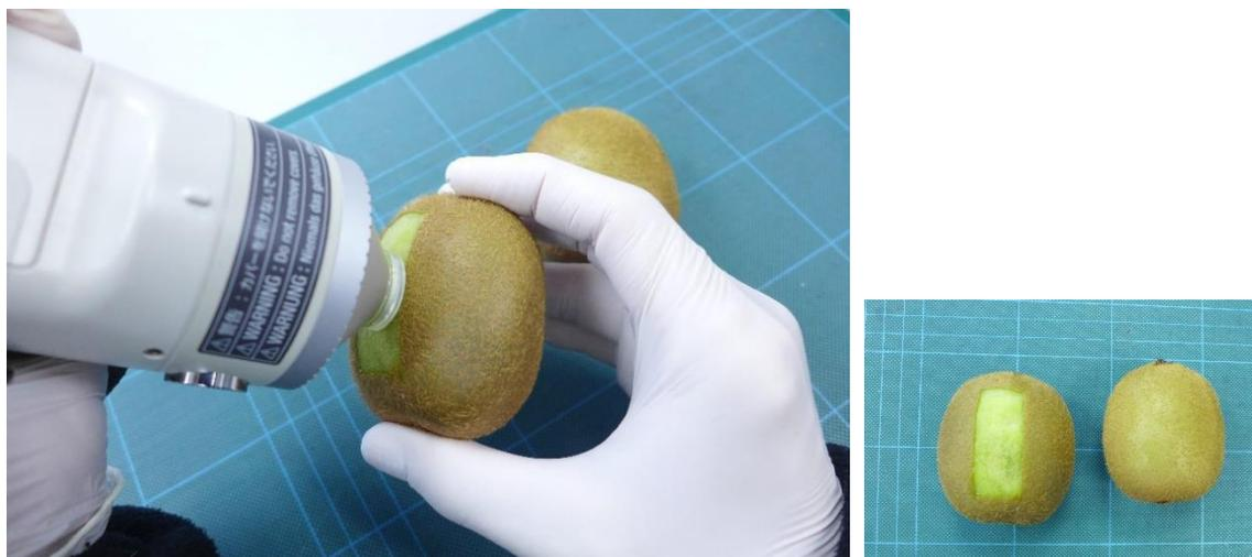
CR-400 employed for the determination of the color of the Kiwifruit (with skin removed) employing the scale CIELAB
