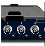
The input modules *labV6* and *labVF6* are 6-channel ICP modules. The *labVF6* is equipped with additional low-pass filters.
