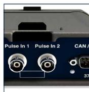
The digital module *labDX* has two CAN inputs respectively one FlexRay input, two Pulse inputs and a AES/RS232 interface for connecting
