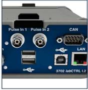
The controller is the central connection unit of a HEADlab system. It is used for data configuration and data concentration.
