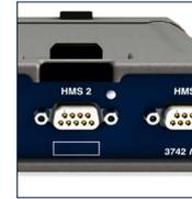
*labHMS* is used for connecting and controlling three digital artificial heads of the HMS III or HMS IV generation.
