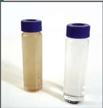
Low-Flow / MicroPurge sampling methods control turbidity and delivery higher quality samples.
